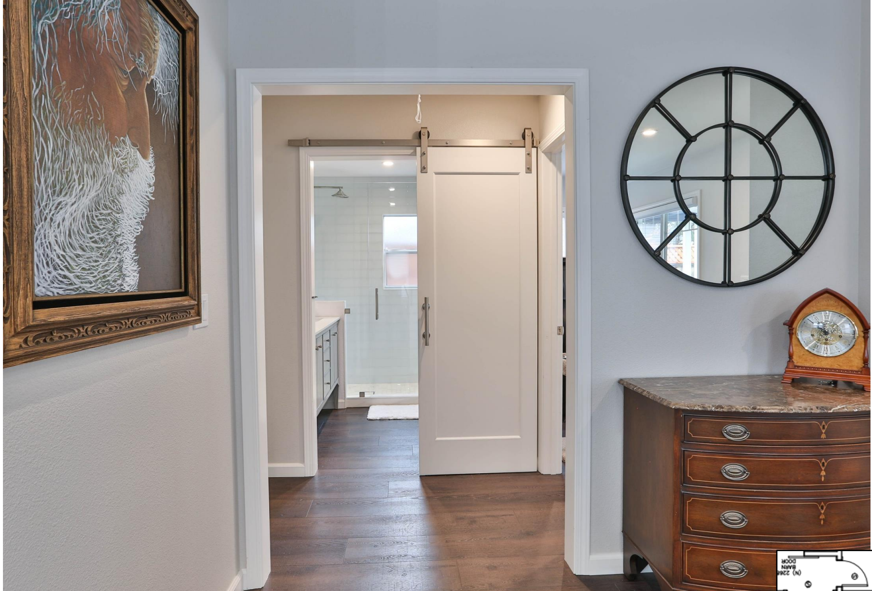
B- AFTER: By eliminating the wall heaters, we were able to widen this hallway opening. We instead installed a mini split heater/ac unit between the family room and kitchen windows. With the help of ceiling fans, evenly conditioned air is felt throughout the tiny house. The hallway closet was absorbed into the bathroom and the bathroom door was relocated and turned into a stylish and space saving barn door. The hallway closet was relocated to the extra space in the living room. (This was cut off of the photograph but is shown on the plans.)
